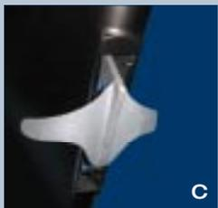
**C.** This carriage is tailored to suit the Ray anchor. It rotates forward and the Ray slides out of it. Most applicable for new builds and can be made to suit any size Ray anchor. A very attractive unit.
